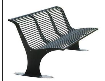
Bench Athena with backrest is totally made of steel. It is composed of two robust laser-cut lateral supports, which are welded to two elliptical bases 600x150 mm. The seat and the backrest are made of steel tubes welded to the lateral supports and of 2 central backings.
